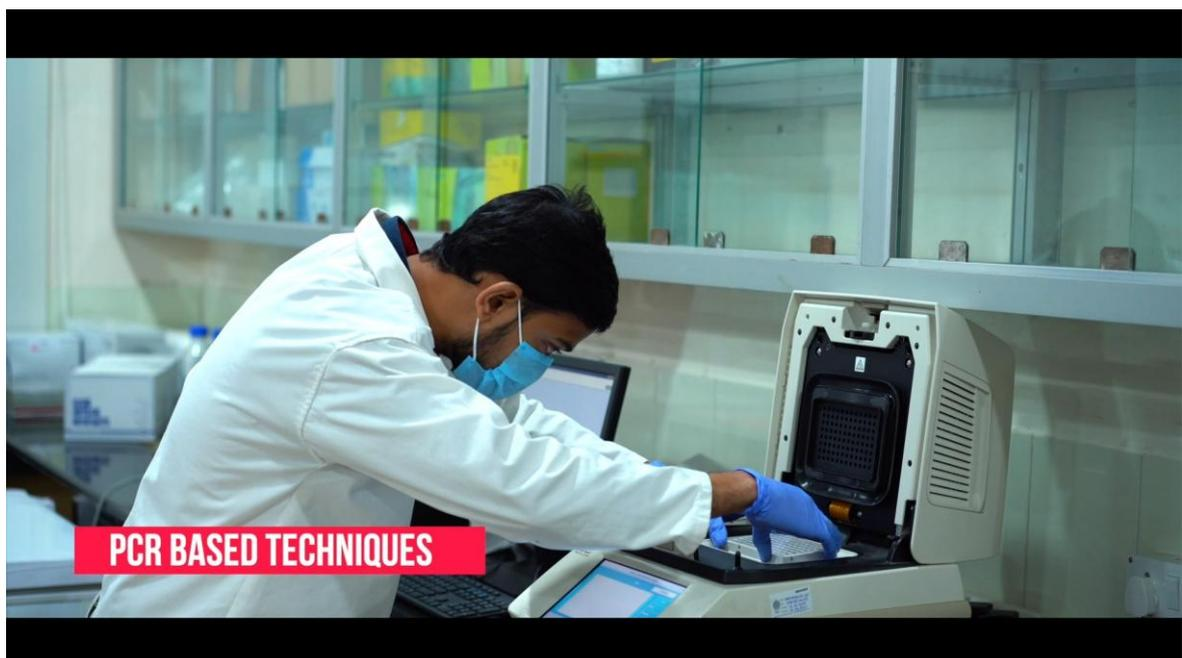
6. End point PCR (Made: Bio-Rad C1000 touch and PegLab version PEQSTAR 2X Gradient).
