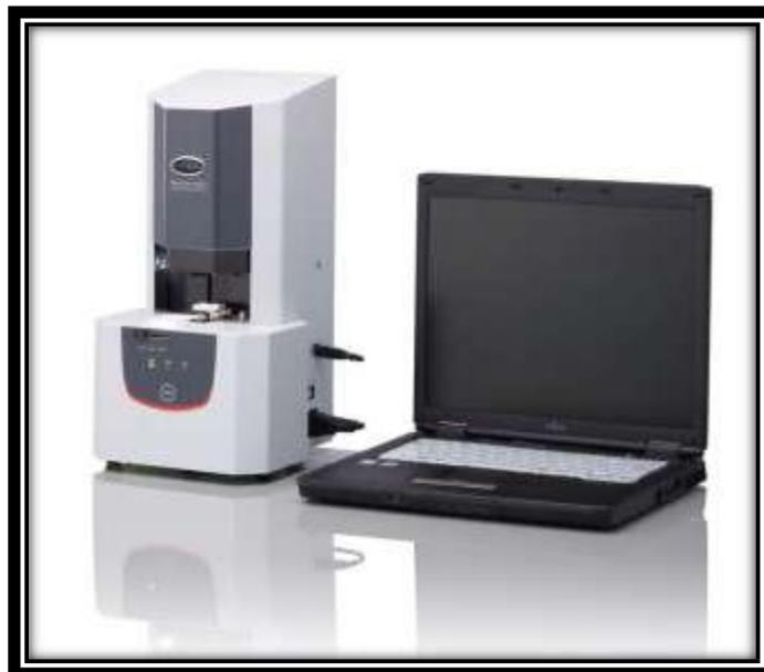
**Principles:** The NanoDrop functions by combining fiber optic technology and natural surface tension properties to capture and retain minute amounts of sample compared to cuvettes or capillaries. Furthermore, the system employs shorter path lengths, which result in a broad range of nucleic acid concentration measurements.
